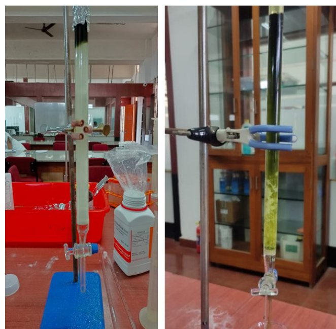
Figure 2. Column chromatography. (A) Packing of the silica column; (B) Running of the sample through the column.
