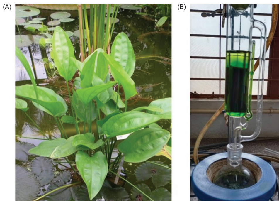
Figure 1. (A) Echinodorus cordifolius ; (B) Extraction of compounds using different solvents by the Soxhlet method.
