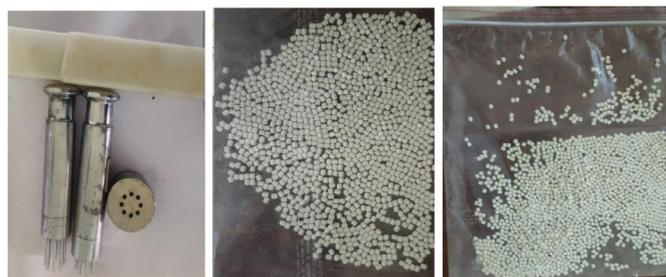
**Figure 5.** Photographic images of the Multi Tip Punches, ER and IR mini-tablets.
