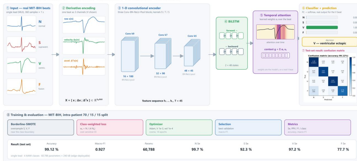
Figure 1: Overview of the proposed derivative-domain CNN-BiLSTM network with temporal attention. A real single-lead MIT-BIH beat is expanded into three channels (raw waveform, first derivative, and second derivative) and passed through a compact three-block one-dimensional convolutional encoder, a bidirectional LSTM, and an additive temporal-attention stage whose learned weights, shown on a real ventricular beat, pool the recurrent states into a beat embedding that is classified into the four AAMI categories. The lower band summarises the training pipeline and the test-set results; the inset softmax probabilities and confusion matrix are the model's actual outputs.
