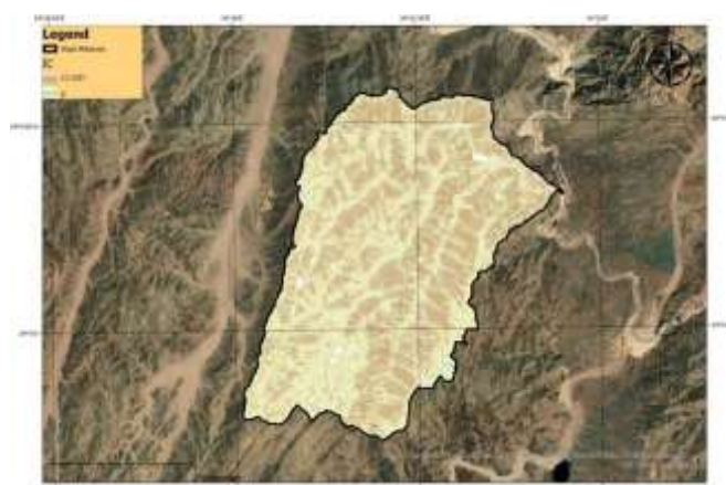
Fig. 23. Index of Connectivity (IC) raster for Wadi Mikeimin (Equation 4, maximum 17.20), combining the upslope and downslope components in Fig. 21 and Fig. 22; higher IC values indicate stronger hydrological connection between hillslopes and the channel network.
