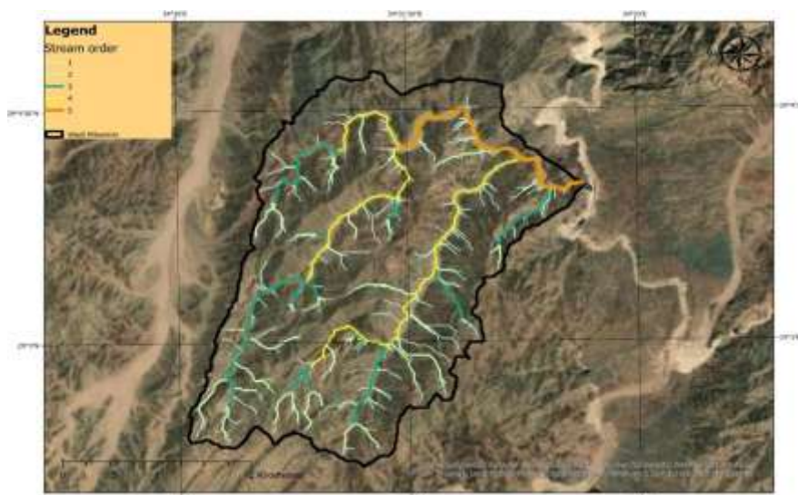
Fig. 8. Strahler stream-order classification in Wadi Mikeimin; higher-order channels (orange) mark the main trunk streams where flow, and hence sediment-transport capacity, is greatest.
