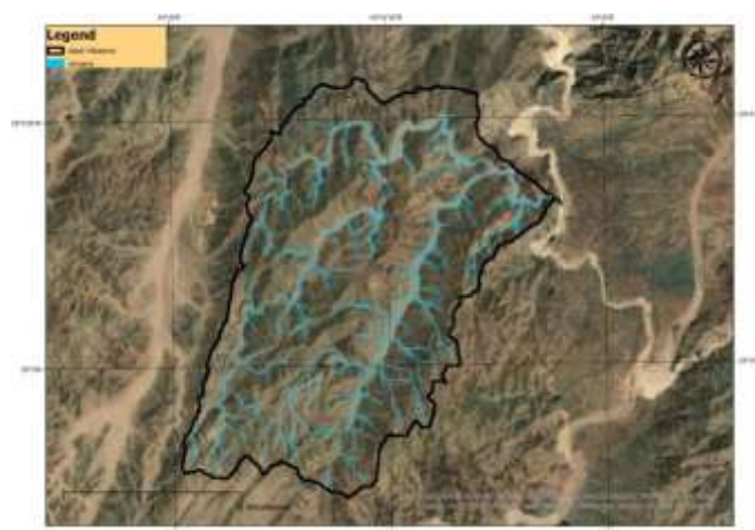
Fig. 7. Drainage network of Wadi Mikeimin delineated from the DEM at a 200 m 2 flow-accumulation threshold, showing the dendritic pattern that concentrates flow toward the single outlet near Nuweiba City.
