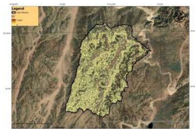
Fig. 25. Final sediment-yield (SY) raster for Wadi Mikeimin (Equation 2, maximum 5.99 \text{ t ha}^{-1} \text{ h}^{-1} for the 100-year design event), obtained by combining the RUSLE soil-loss map with the Sediment Delivery Ratio; the pattern closely follows the main drainage network.
