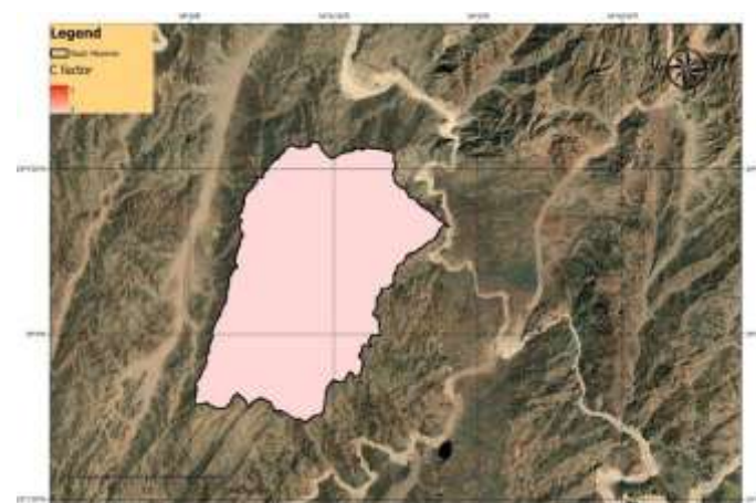
Fig. 16. C-factor (cover-management) raster for Wadi Mikeimin; the near-uniform value of 1 reflects the catchment's near-complete bare-ground land cover.
