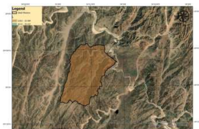
Fig. 14. L-factor (slope-length) raster for Wadi Mikeimin, computed from flow accumulation and cell size via Equation (14).
