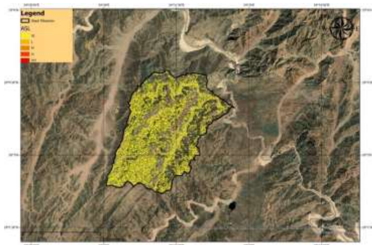
Fig. 20. Soil-loss severity classification (Table 6) mapped across Wadi Mikeimin; the catchment falls predominantly within the very-low-to-low erosion classes, with isolated higher-severity cells along steep channel margins.
