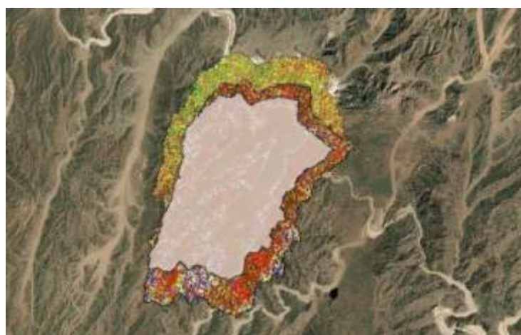
Fig. 18. Composite RUSLE soil-erosion map for Wadi Mikeimin, combining the R, K, LS, C and P rasters (Equation 1); the highest soil-loss values are concentrated along the steep catchment margins.
