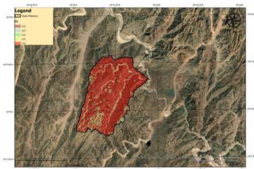
Fig. 13. Spatial distribution of the LS-factor exponent m in Wadi Mikeimin, reclassified from the DEM-derived slope grid into the ranges m = 0.2\text{--}0.6 .
