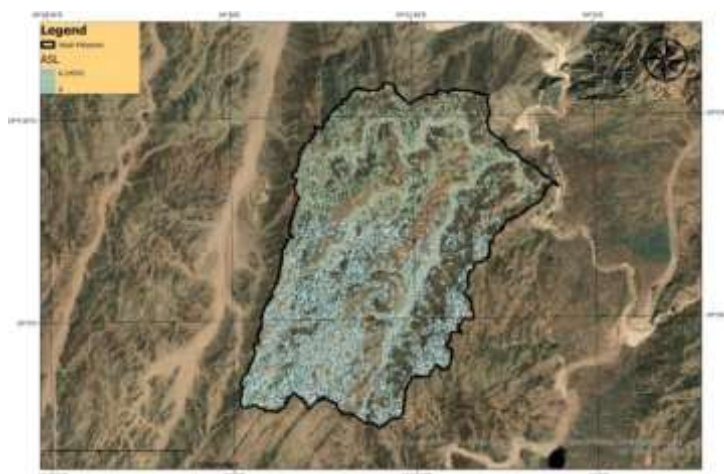
Fig. 19. Gross soil-loss (A) raster for Wadi Mikeimin ( \text{t ha}^{-1} \text{h}^{-1} , maximum 6.25), overlaid on the catchment boundary.
