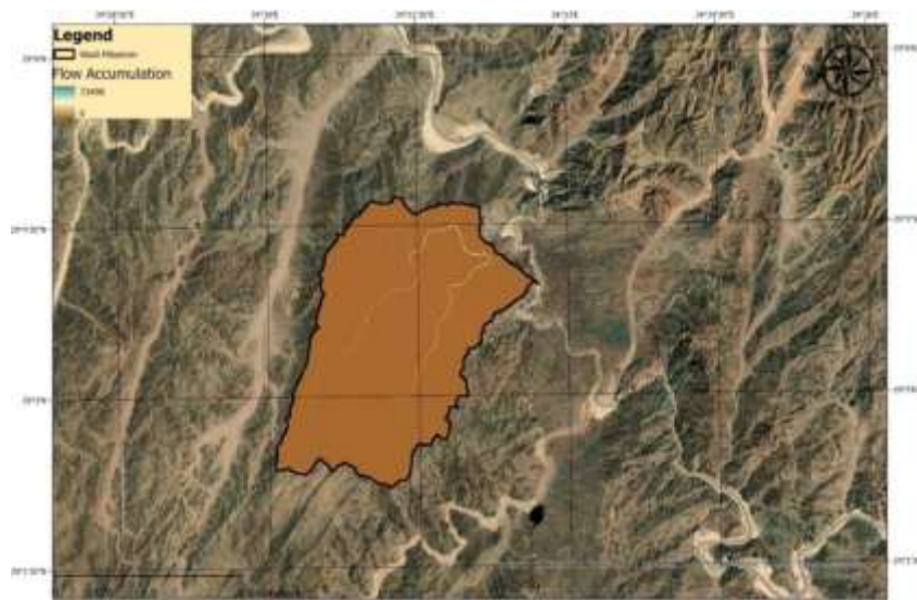
Fig. 12. Flow accumulation rates from the DEM, computed in ArcGIS Pro.
