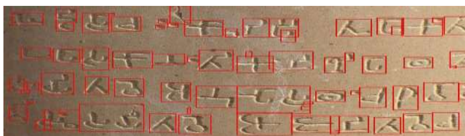
Figure 18: Bounding box for UNet VGG by applying contour plotting over the mask generated by the CNN model
