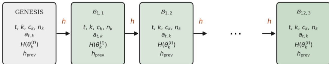
Figure 8: Structure of the SHA-256 audit chain. Each block records the round index, client and cluster identifiers, shard size, local accuracy and a digest of the submitted parameters, together with the digest of its predecessor. Thirty-six blocks are produced over twelve rounds with three clients.
