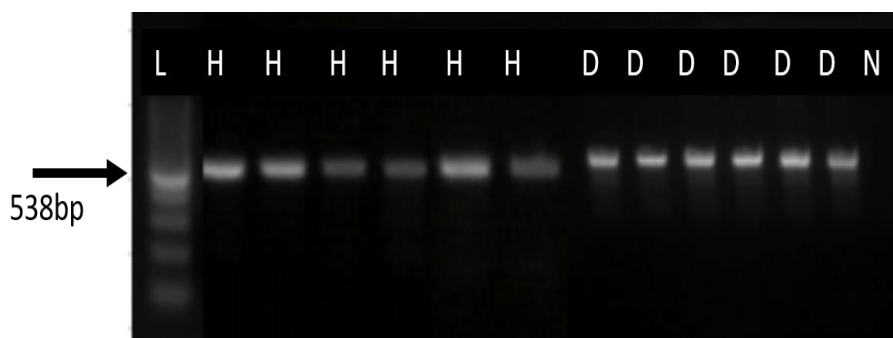
Fig. 3: L: 100bp Molecular marker, PCR products (538bp) for samples, H: Cardiovascular Disease, D: Diabetes, N: Negative control
